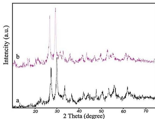
**Fig. 1** – XRD pattern of as prepared samples at: (a) without ultrasound (sample No1), (b) power of ultrasound 75 W (sample No 3)
