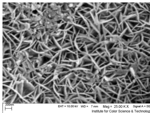
**Fig. 5** – SEM images of samples obtained under hydrothermal condition: 90 °C for 10 h
