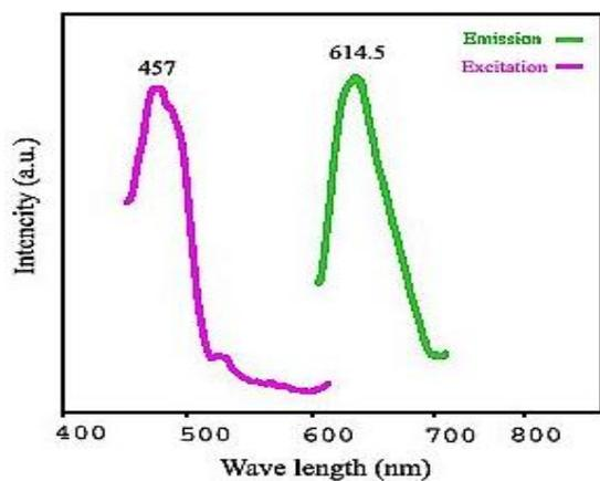
**Fig. 3** – The room-temperature photoluminescence spectrum of the nanostructure  $\text{NiMoO}_4$ . (sample No 3)
